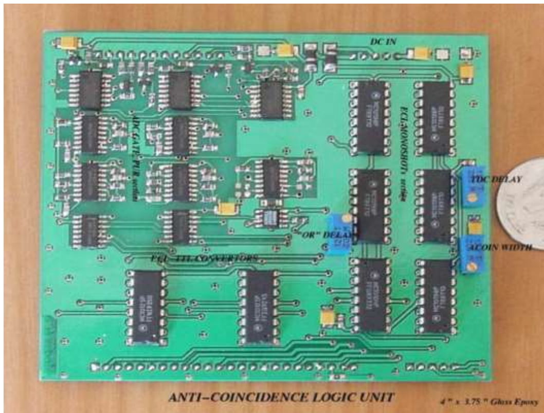
Fig: ACLogic card with typical signals monitored
