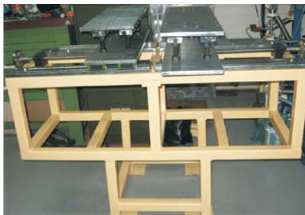
Fig.8. Alignment/mounting structure fabricated at IUAC
