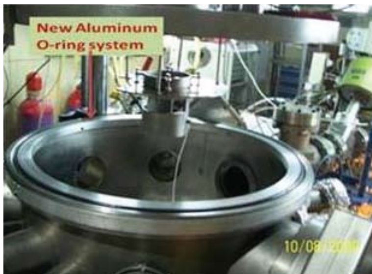
Fig. 1. Irradiation chamber with new o-ring system
