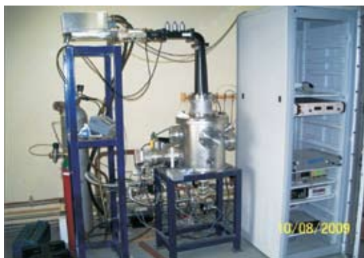
Fig. 2. Microwave plasma system for thin film deposition
