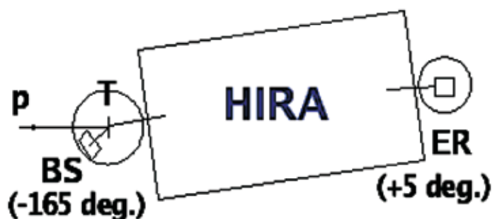
Fig.1. Kinematic coincidence setup showing the mean angles for projectile-like and target-like particles
