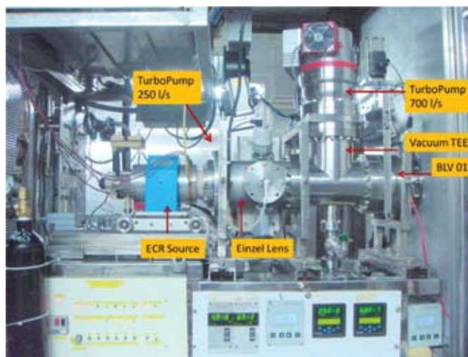
Fig. 1 : HV Deck Components after modification
