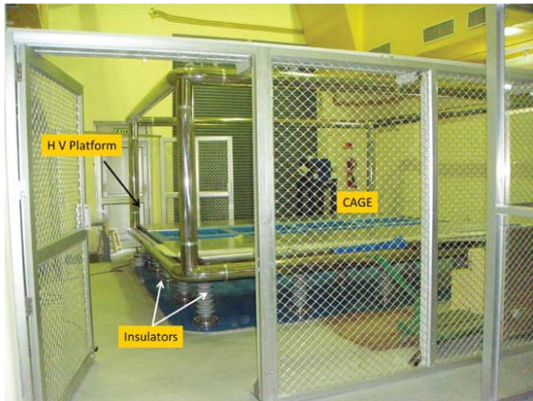
Fig. 3 : High Voltage Platform and Cage in Beam Hall
