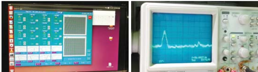
Fig. 2.2.2 (left) View of the VME based control system; (right) view of the beam at the first beam profile monitor after the analyzing magnet.
