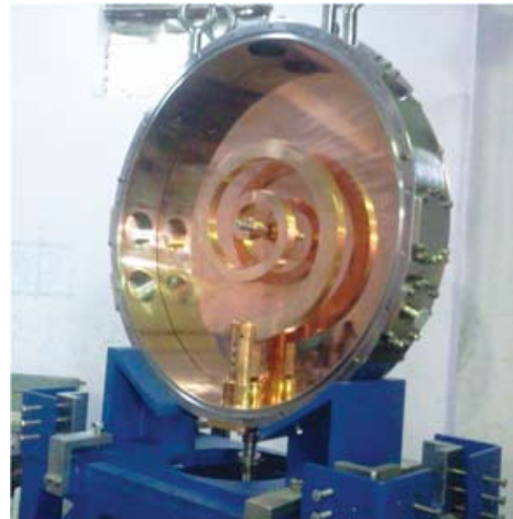
Fig. 2.2.10 Final design parameters for the spiral buncher
