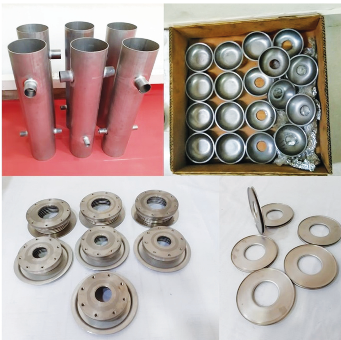
Figure 1: Clockwise from top-left: (i) niobium housings, (ii) end caps and upper caps, (iii) welded niobium leaves for the slow tuner bellows, (iv) transition flange assemblies.
