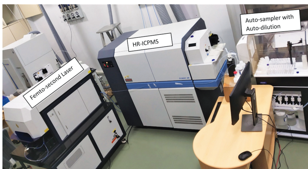
Fig 2: HR-ICPMS installed with Femto-second laser, auto-sampler and auto-dilution system
