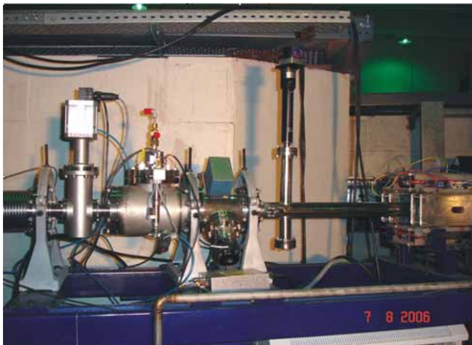
Fig. 1. The beam line with cross for equilibrium charge state studies mounted
