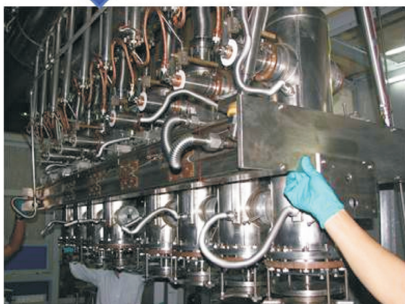
Figure 1. Three accelerating modules and the second cryostats with eight resonators of LINAC
