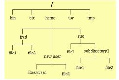
Figure 1.2: The GNU/Linux file system tree.
