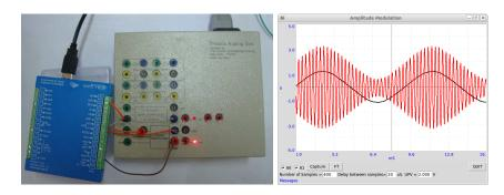
Figure 5.11: Amplitude modulation.(a) Experimental setup (b) Modulating signal along with the modulated output.
