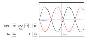
Figure 5.3: Inverting Amplifier making 1800 out of phase sine wave.
