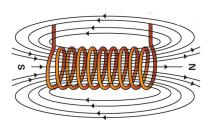
Figure 3.4: (a) Current carrying solenoid repelling a permanent magnet. (b)Magnetic field of a current carrying solenoid
