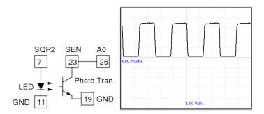
Figure 5.10: The waveform at the photo-transistor collector
