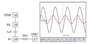
Figure 2.14: Screenshot showing the total voltage across the RC circuit and the voltage across the capacitor. C=1 uF and R =  $560\Omega$ .
