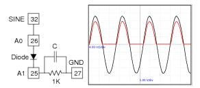
Figure 5.1: Diode as a half wave rectifier.
