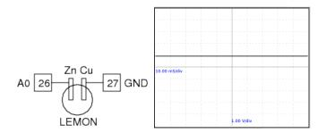
Figure 2.3: (a)Copper and Zinc plates inserted into a Lemon. (b) The DC voltage output from the cell.
