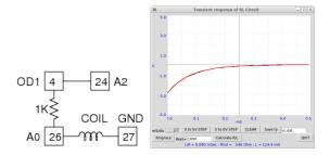
Figure 2.11: LR circuit. Voltage across the inductor after a 5 to 0V step.
