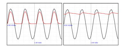
Figure 5.2: Rectifier with Filter. (a) 1 uF (b) 100 uF.
