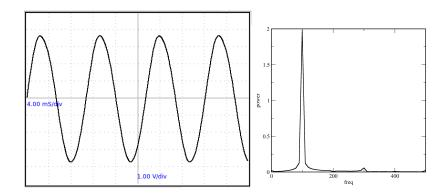
Figure 2.20: (a) Sine wave. (b) Frequency spectrum by Fourier transform.
