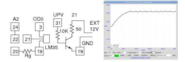
Figure 6.5: Temperature measurement using LM35.
