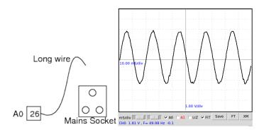
Figure 2.6: Power line pickup
