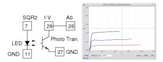
Figure 5.9: CE characteristic of photo-transistor.
