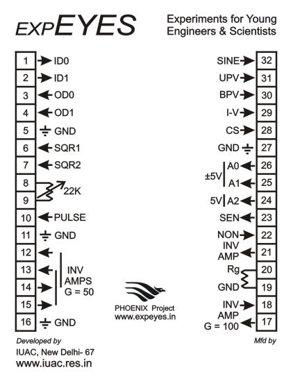
Figure 1.1: The ExpEYES top panel showing the external connections on both sides. The arrows indicates the direction of the signals..
