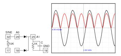
Figure 5.4: Full wave rectifier using two diodes.
