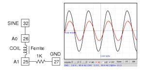
Figure 2.17: LR circuit. Effect of Ferrite core.
