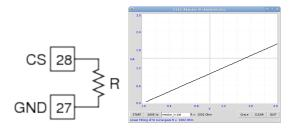
Figure 2.2: IV-characteristic of resistor
